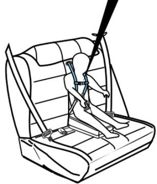
8. Pull the shoulder belts toward you to make sure the crotch safety belt buckle is properly fastened and the retractor is locked.
